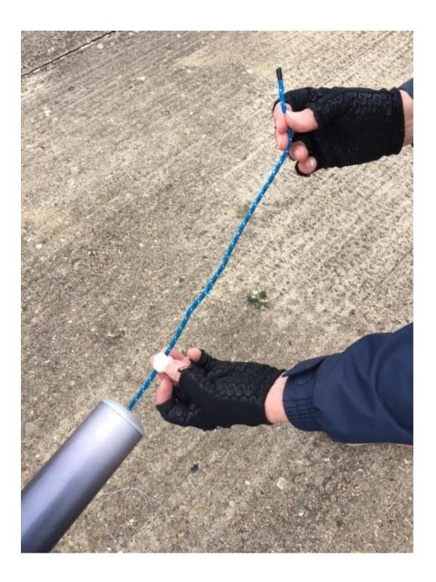
8. Make a new external stopper knot (technically a double overhand knot) approximately 200mm from the end of the pole when the rope is pulled forwards as far as it will go. Any less than this, and the gennaker won't go far enough back into the sock during drops. But too large a gap between the internal and external knots will result in the kite flying too far to leeward.
