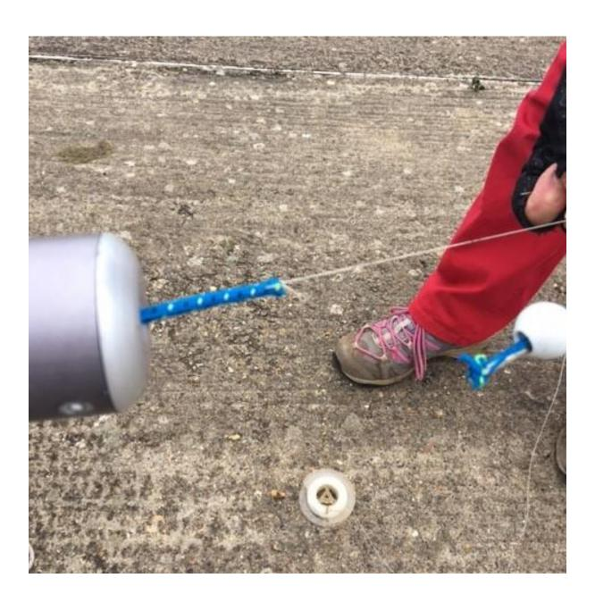
2. Carefully reach through the hole at the back of the pole with a hook, a little finger, or a pair of surgical scissors, and withdraw a loop of the internal rope.
