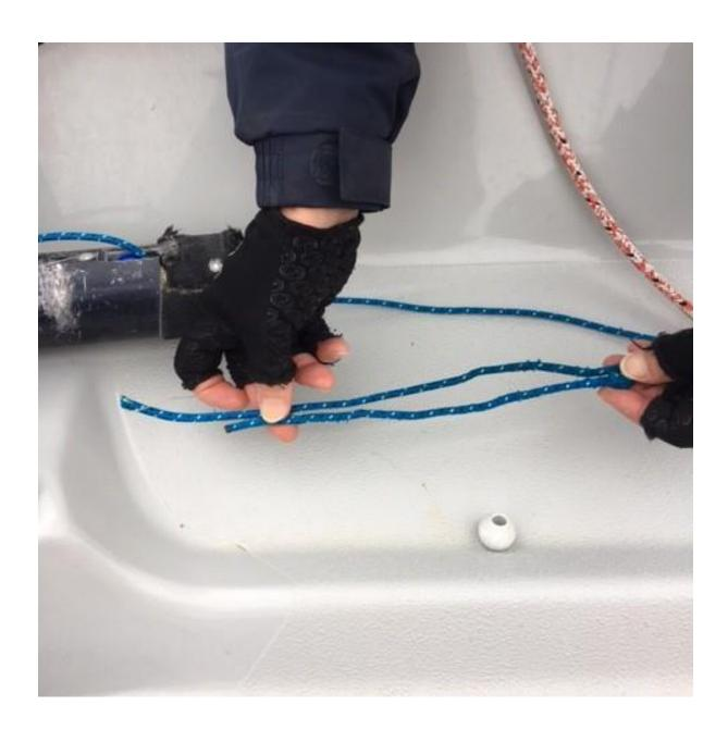
5. Lay out the old piece(es) of rope in order to judge where to make the new internal knot, allowing about 60 mm extra (about 5 dyneema speckles as shown above) to allow for the new external stopper knot.
