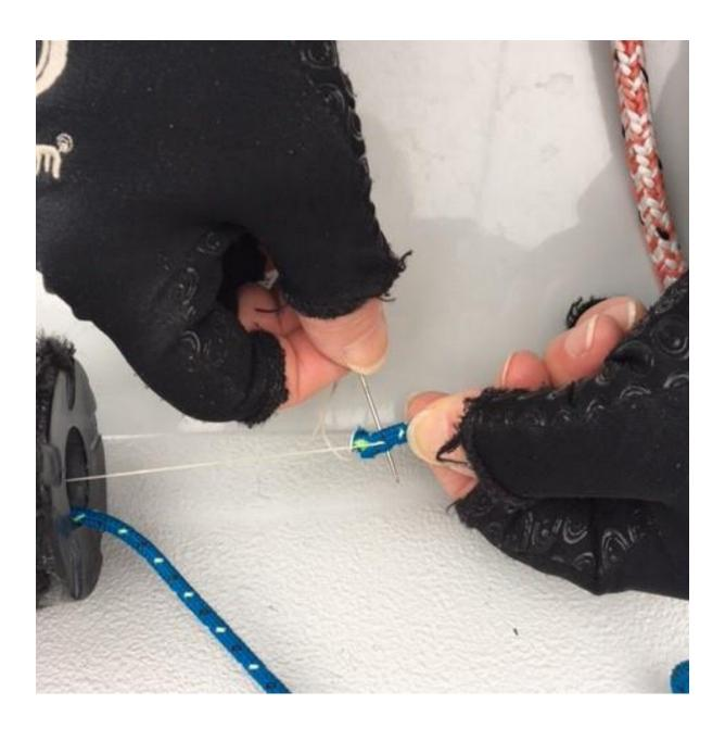
6. Feed the end of the rope back inside the pole. It helps if someone else can simultaneously pull gently and steadily on the keeper line at the front of the pole to maintain tension.
